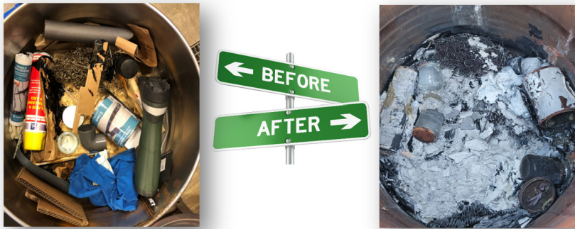
Figure 1 - Waste before and after applying inDRUM technology.
