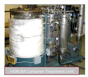
The inDRUM process consists of two main treatment systems. An in-container autoclave treatment system which vaporizes liquids, thermally decomposes carbon based compounds, and stabilizes reactive materials, The second system if the off-gas treatment system: consisting of thermal oxidizer, quench scrubber, filtrations systems, and other equipment to achieve the necessary emissions standards.
