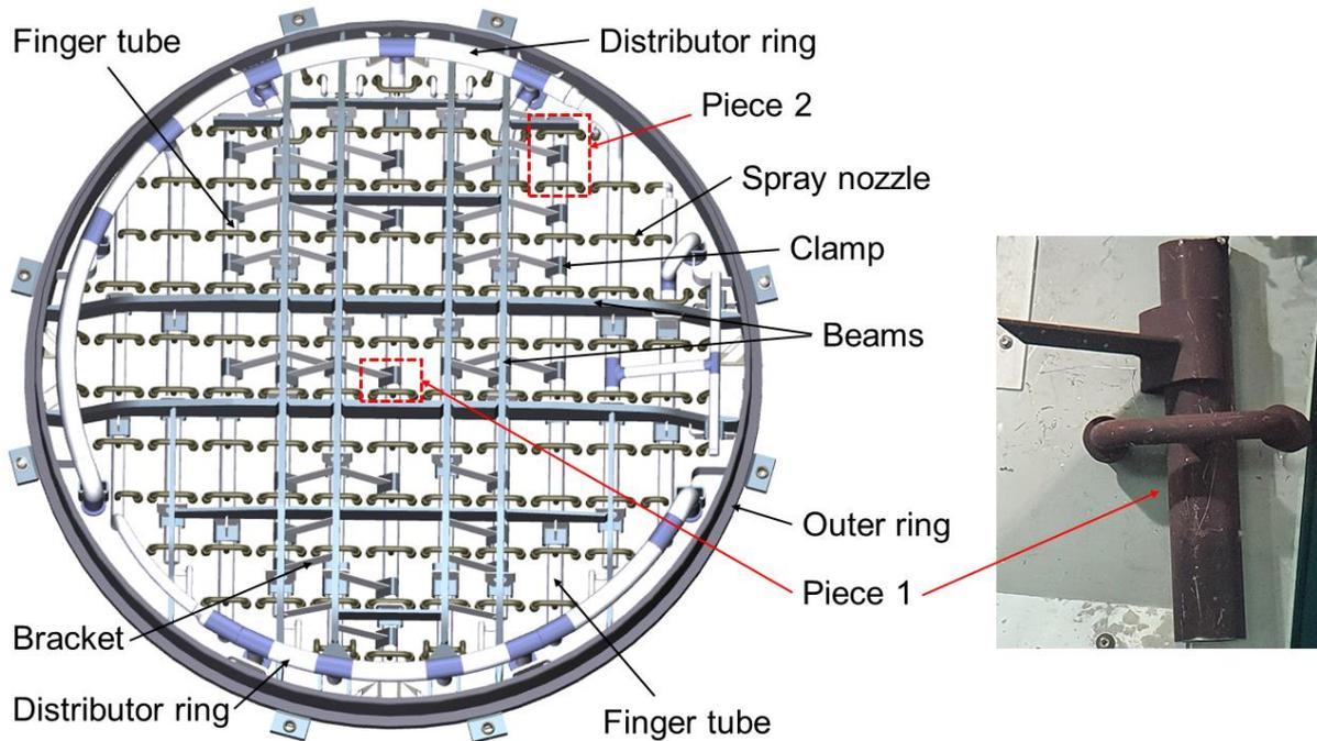
**Figure 4: Schematic of the Oskarshamn 1 core spray system including the locations of Pieces 1 and 2 (left) and a photo of Piece 1 (right).**
