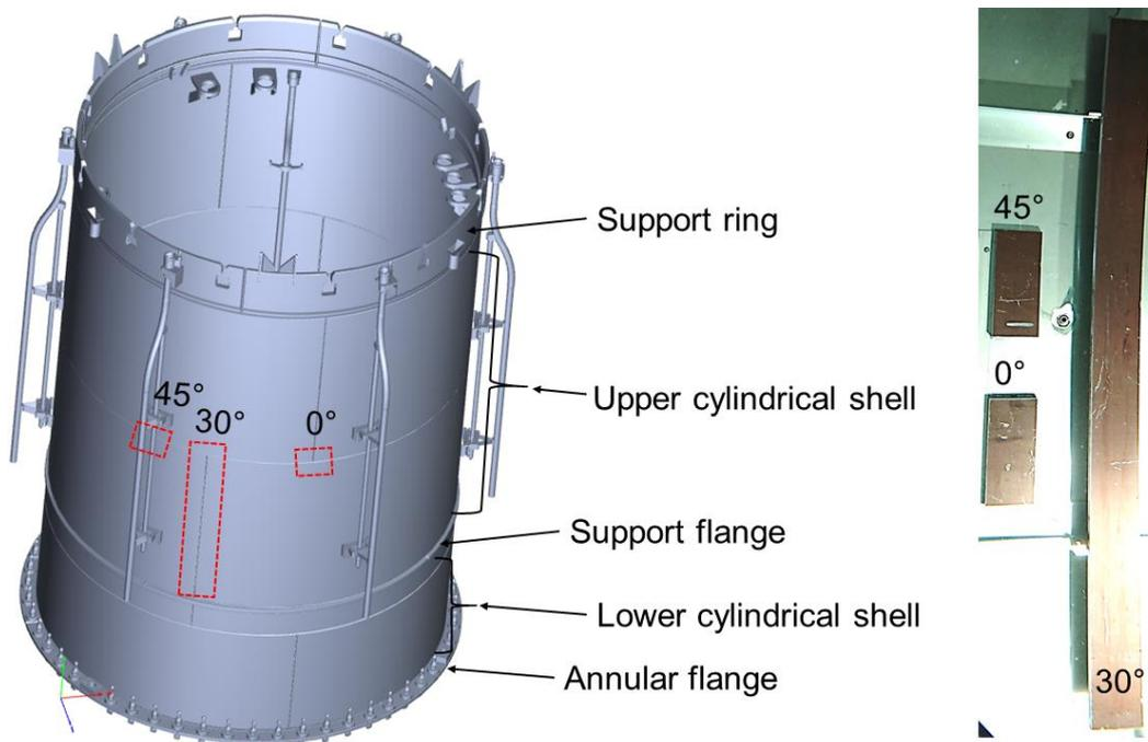
**Figure 1: Schematic of the core shroud from Oskarshamn 2 and the locations of the pieces of material harvested from the component (left), and a photo of the three pieces (right)**
