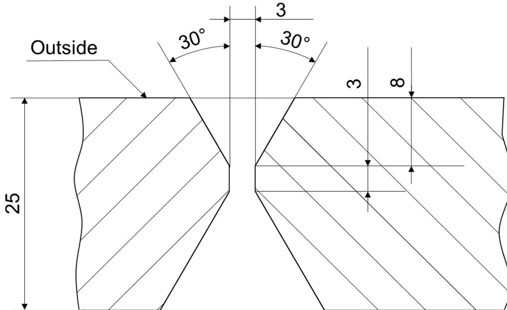
**Figure 2: Schematic of the horizontal and vertical weld geometries in the upper cylindrical shell of the Oskarshamn 2 core shroud**
