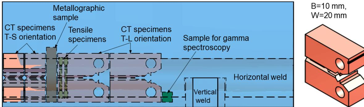
**Figure 6: Schematic showing the samples and specimens machined from the piece located at 30° and the CT specimen to be used for fracture toughness testing. The horizontal dashed lines indicate the weld fusion lines**
