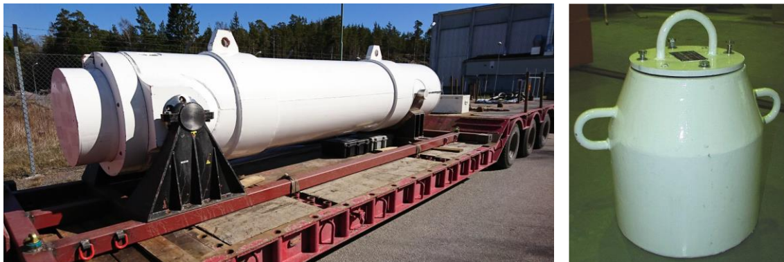
Figure 2: Transport casks Type A – 29 tons, Ø450 mm × 4 m (left), Ø300 mm × 450 mm (right).
