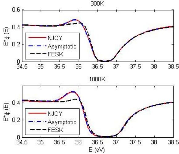
Fig. 2. Neutron spectrum at  $^{238}\text{U}$  36.68 eV resonance
