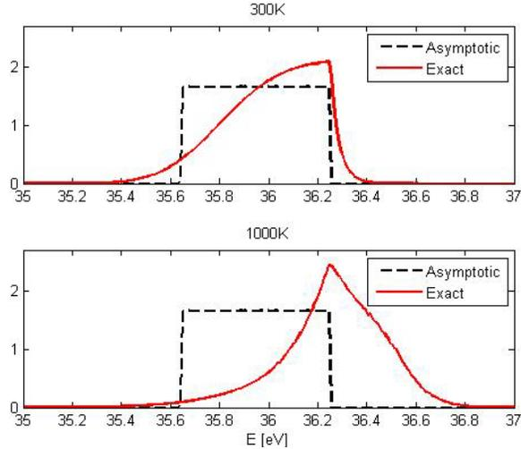
Fig. 1.  $^{238}\text{U}$  scattering kernels at 36.25 eV
