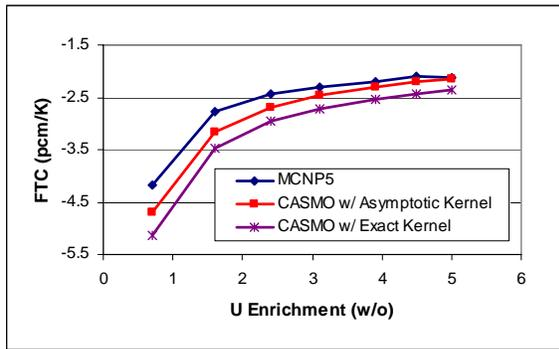
Fig. 3. Fuel temperature coefficients of UO<sub>2</sub> pin
