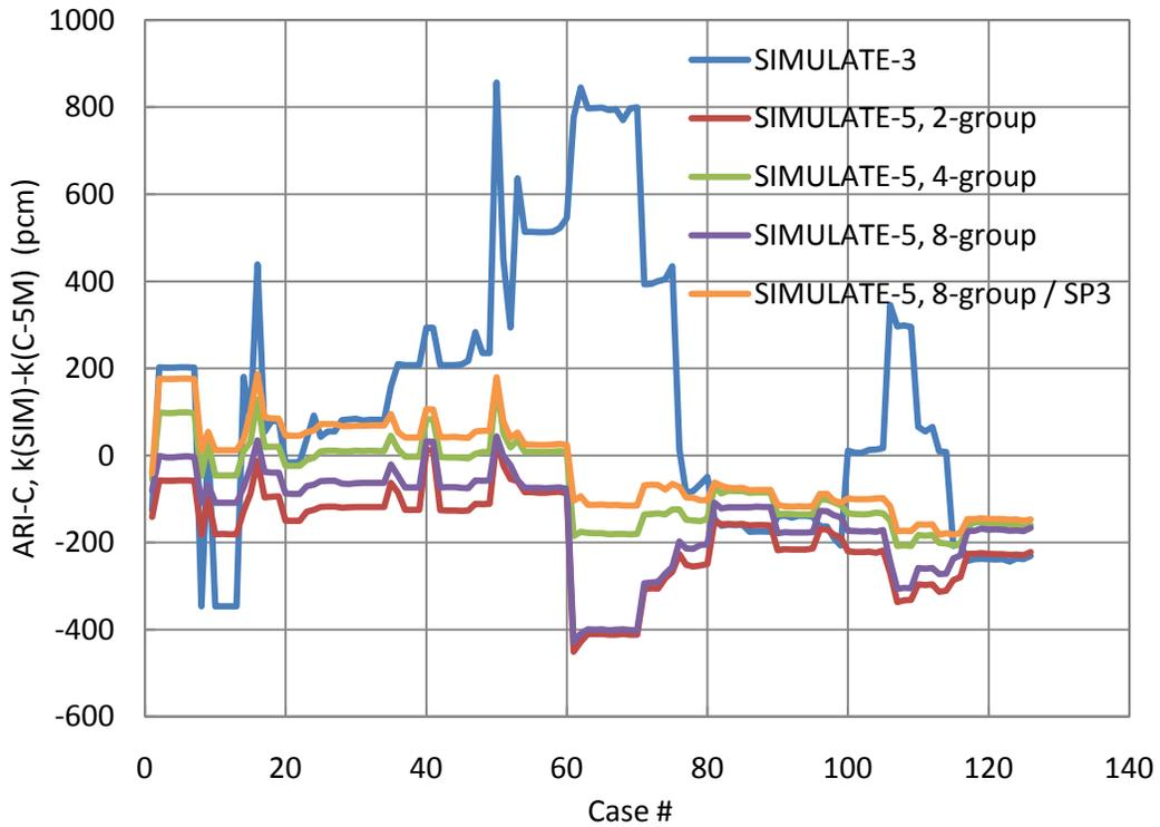
**Fig. 6** SIMULATE-3/5 vs. CASMO-5M benchmark result for the ARI-C case.
