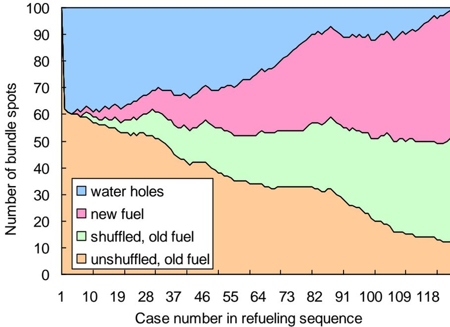
**Fig. 2** Fuel bundle types during refueling in the 10×10 mini core.
