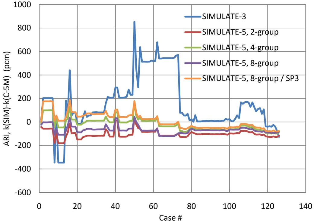
**Fig. 5** SIMULATE-3/5 vs. CASMO-5M benchmark result for the ARI case.
