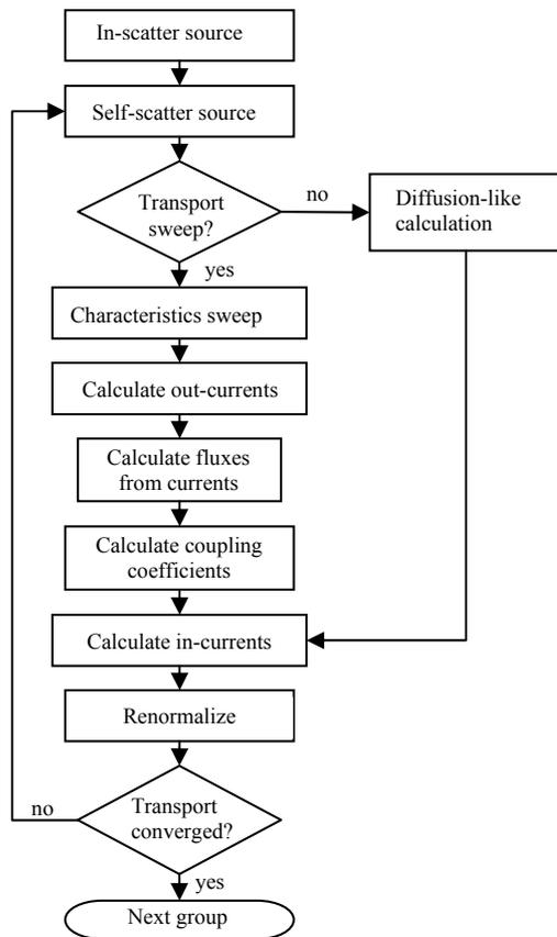
Figure 1. The calculation scheme for the MOC transport solver in HELIOS-2.
