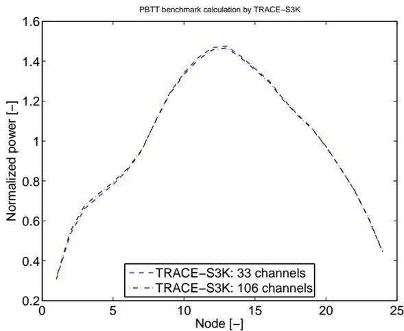
**Figure 10. Initial core axial power profile for 33- and 106-channels models**
