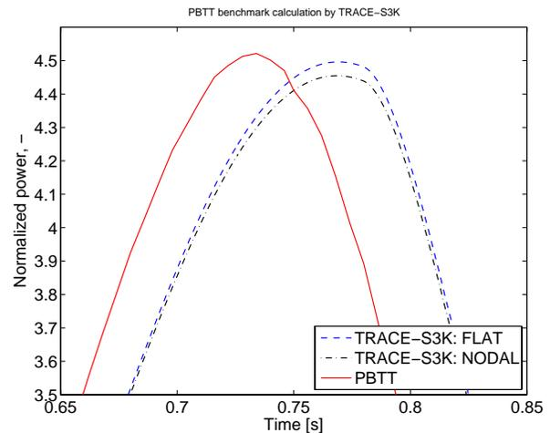
**Figure 9. Relative power for different coupling options**
