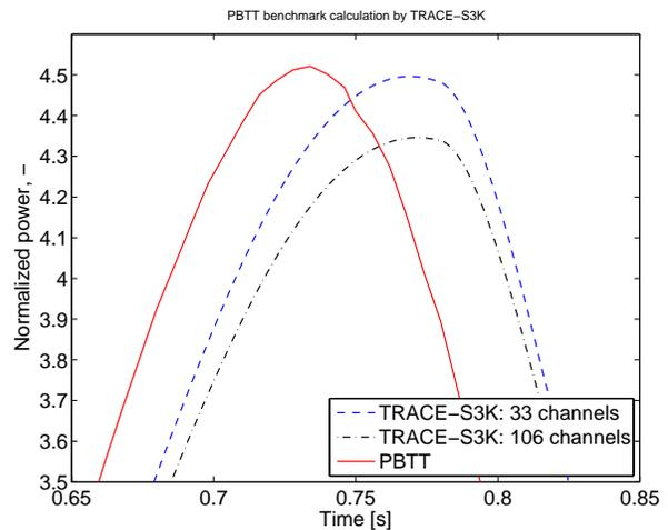
**Figure 11. Relative power for 33- and 106-channels models**
