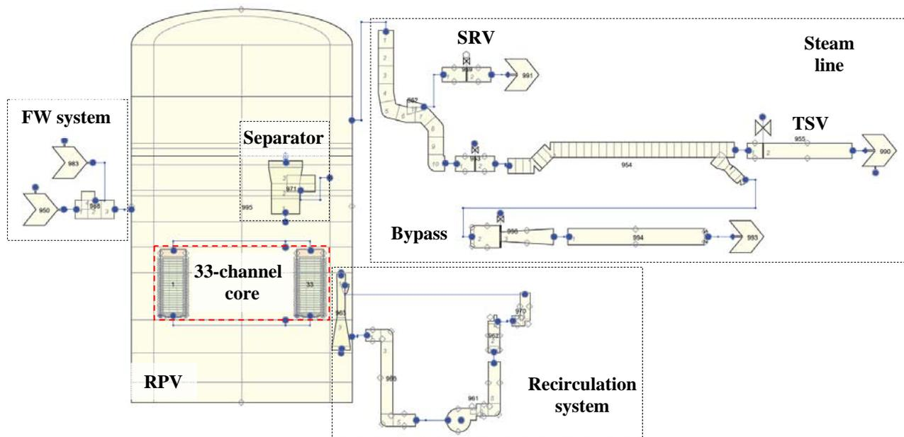
**Figure 1. Schematic TRACE model for PB2 TT2**
