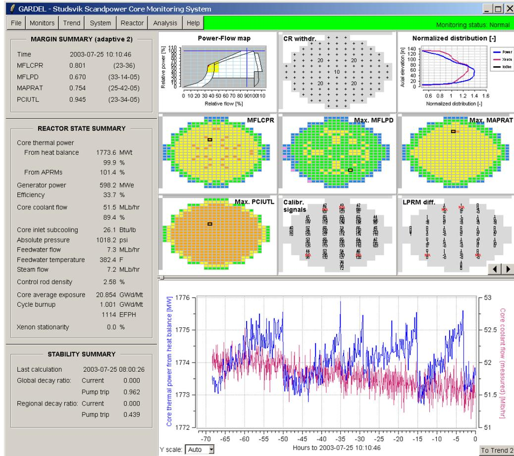
This information includes global reactor data with overall thermal margins core stability and reactor statepoint conditions, trend plots for core scalar values (both calculational results and process signal data, core radial maps of the most important current online distributions, measured and predicted LPRMs signals, the current power flow map with showing the last 72 hours of operation and core average power and fission product distributions.
