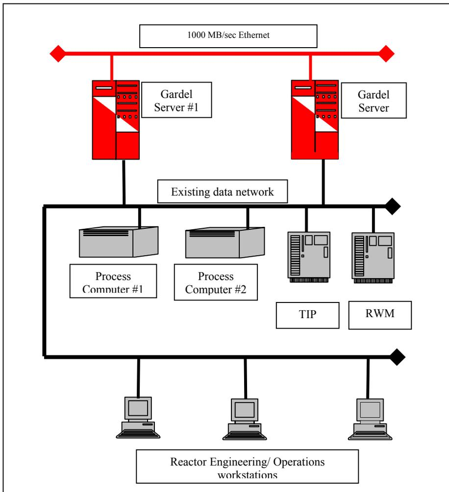
The GARDEL-BWR system is designed to be independent of the underlying hardware and operating system by using standard FORTRAN programs for the computationally intensive processes and uses the TCL/TK language for graphical interfaces that are used to display results and serve as the graphical user interface (GUI). The system has been ported to a variety of UNIX based (Sun, HP, Linux) systems and Windows 2000 Server platforms.
