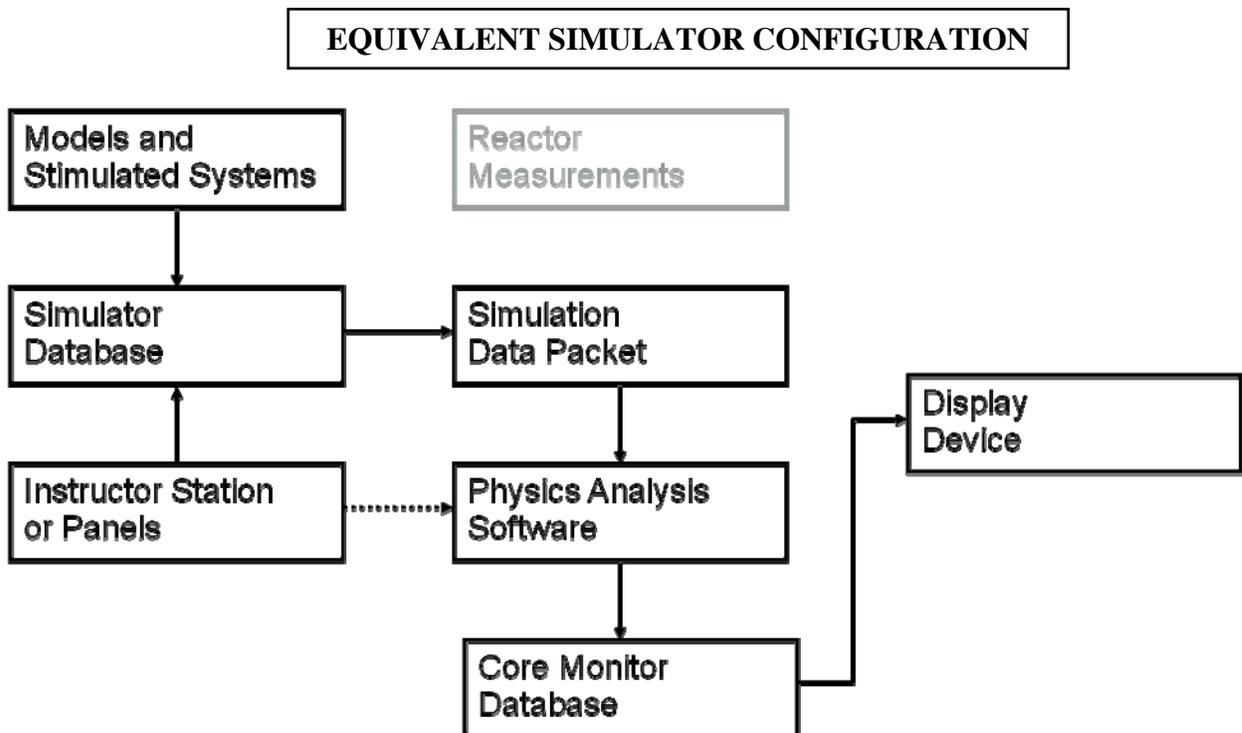
Fig. 1 GARDEL and GARDEL-SIM Configurations
