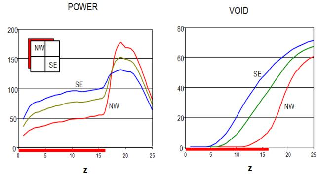
**Fig. 2. SIMULATE5 power & void distribution with QTH option**
