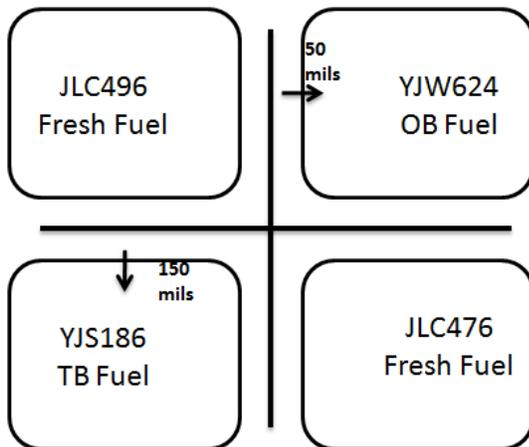
Fig. 3. Control cell with an assumed channel bow
