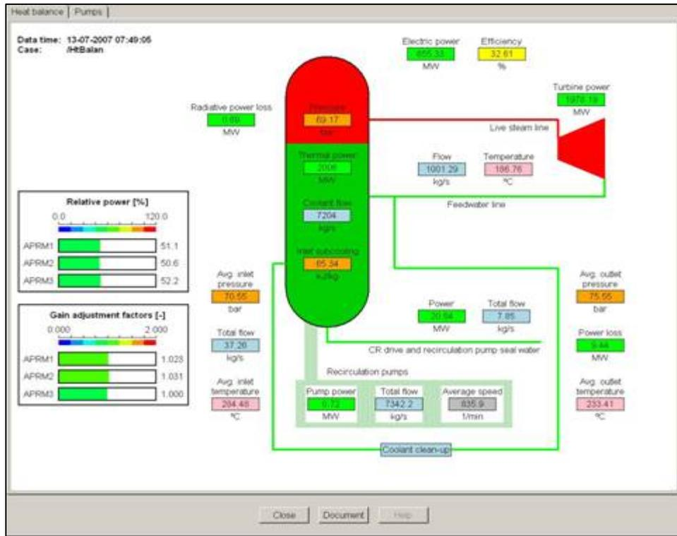
Fig. 1 Example of BWR heat balance mimic display.
