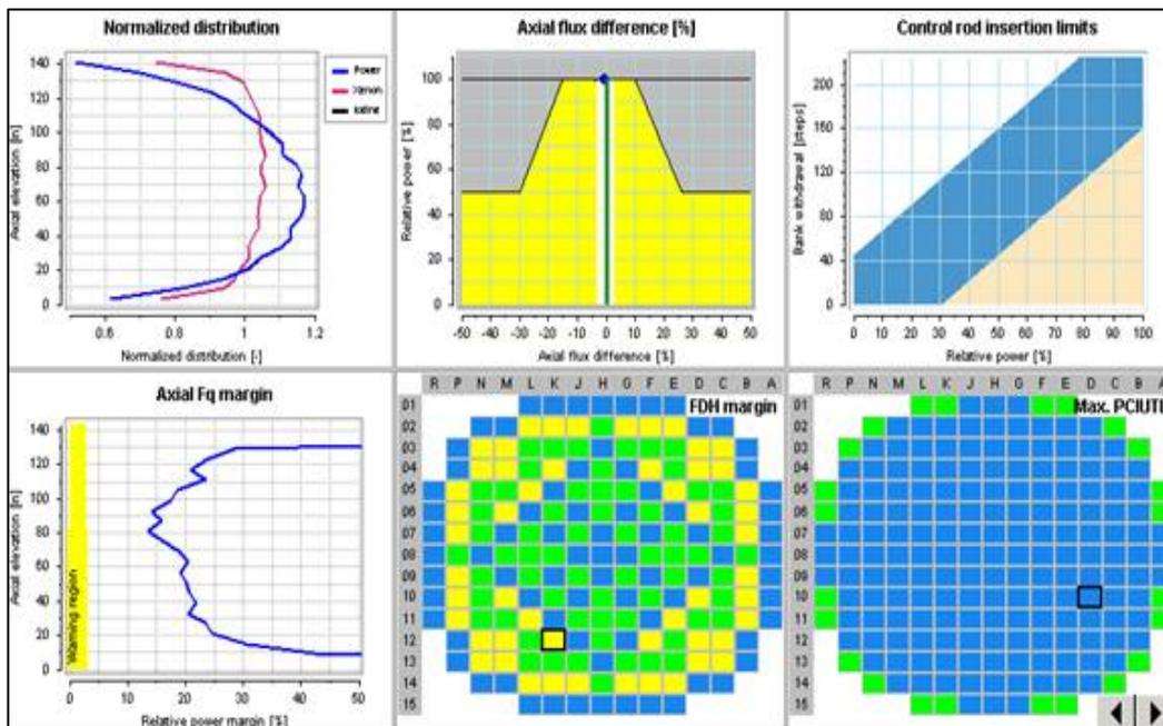
Fig. 2 Example of PWR on-line monitors
