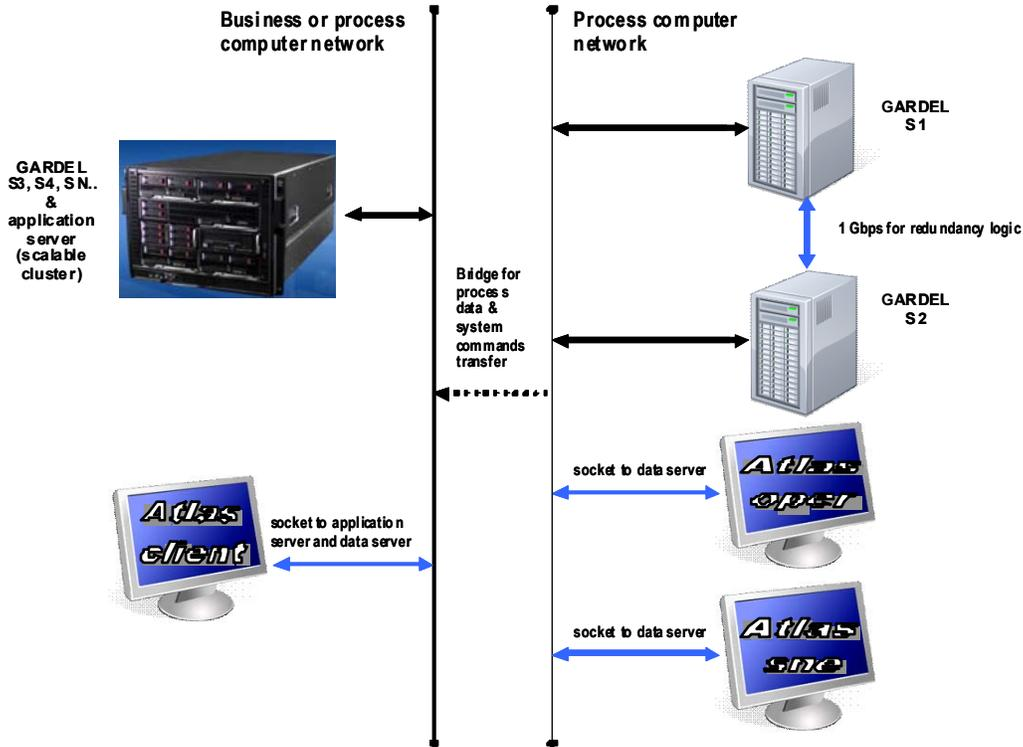
Fig. 5 Recommended GARDEL configuration
