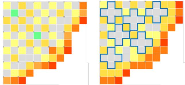
Fig. 6. Equilibrium Cycle, 152 Fresh Loading Reference vs. ACCD
