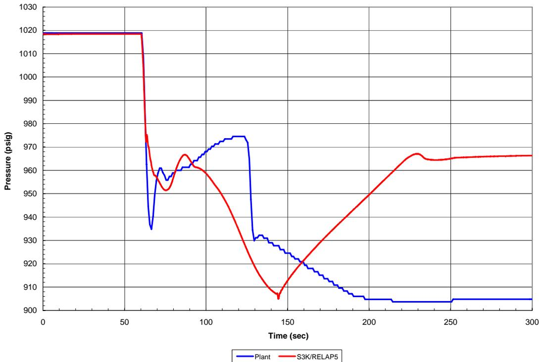
Fig. 2 Reactor pressure for the manual scram.
