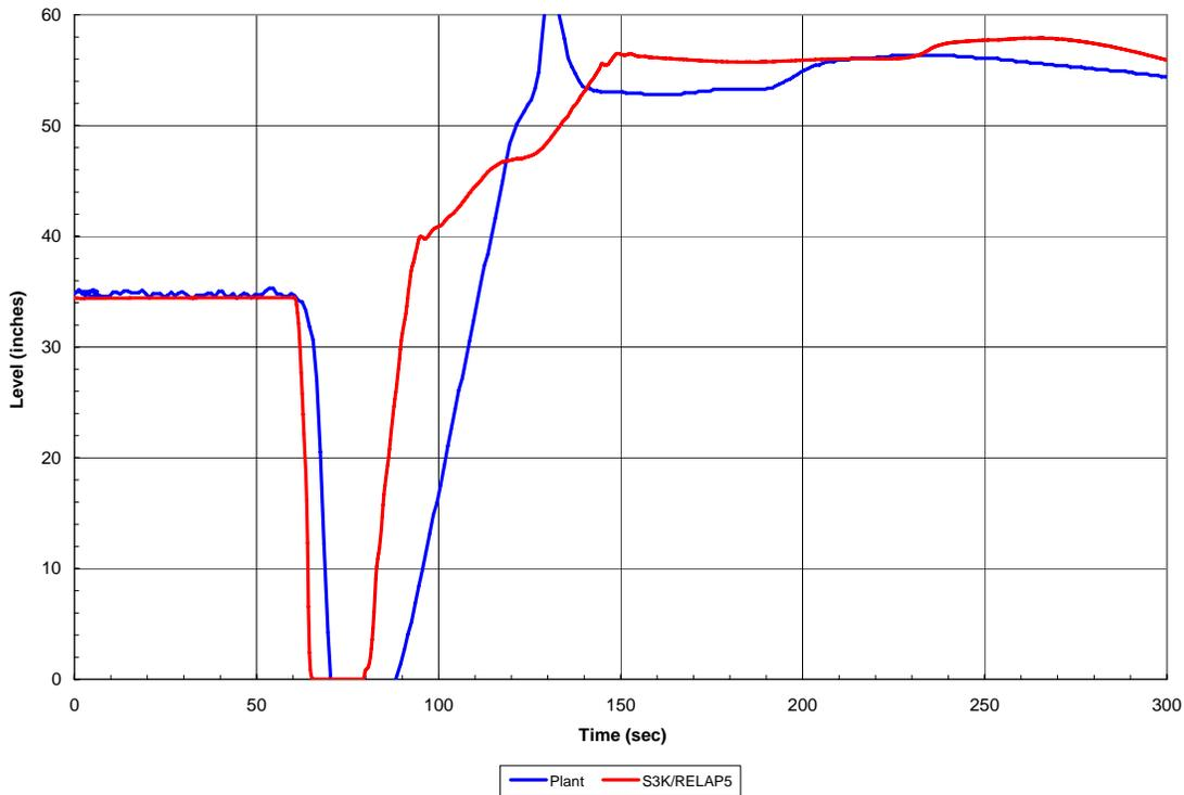
Fig 3 Reactor level for the manual scram.
