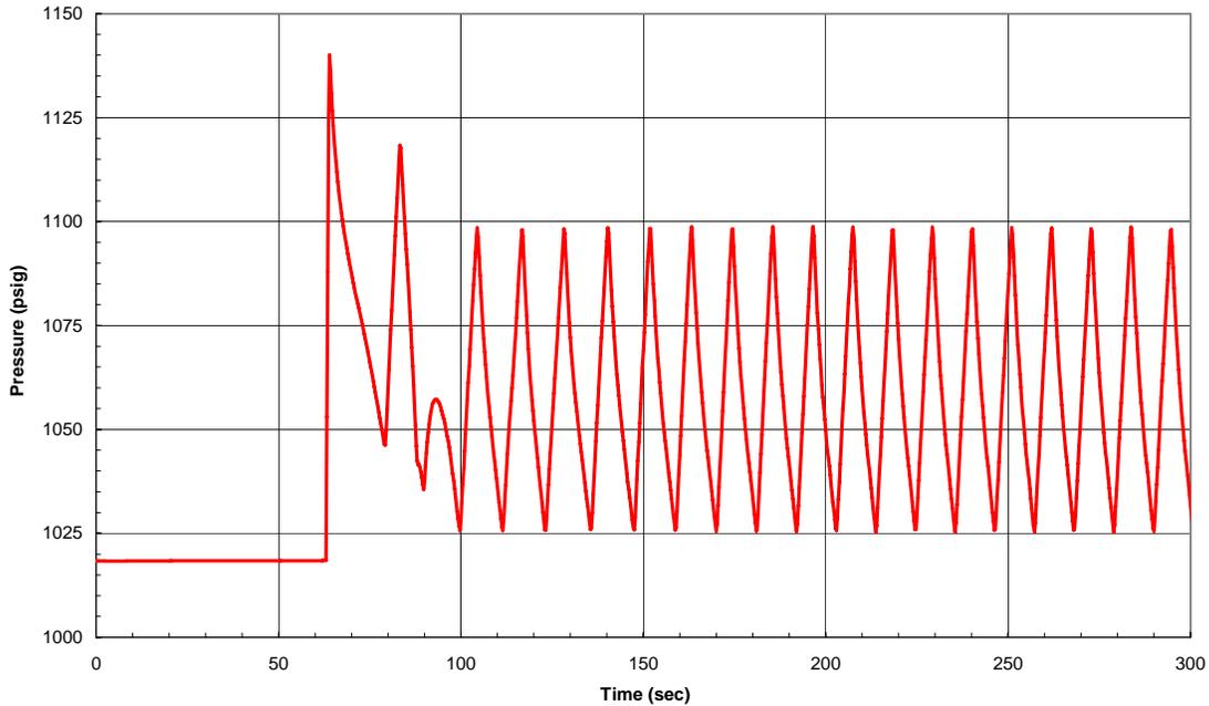
Fig. 7 Reactor pressure for the MSIV-ATWS transient
