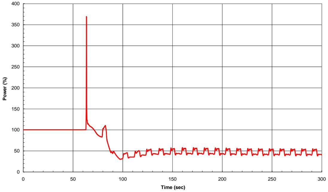
Fig. 5 Reactor power for the MSIV-ATWS transient.
