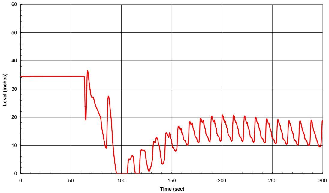
Fig. 6 Reactor water level for the MSIV-ATWS transient
